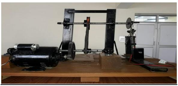
This machine consist power transmission system and SCOTCH YOKE MECHANISM. Power transmission system transfer power from motor to final shaft on which scotch yoke mechanism is installed, this mechanism convert rotatory motion into reciprocating motion. A punch is connected to scotch yoke mechanism which compresses the molten plastic material into the die through nozzle. After solidification desired product is obtained.
